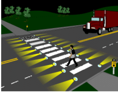
Figure 2 In-Pavement Warning Lights System (5).
